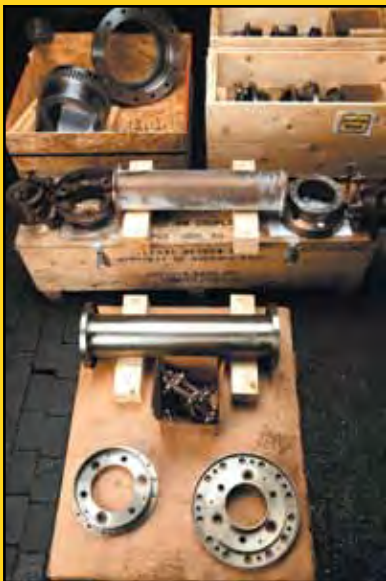
High performance coupling for refurbishment
