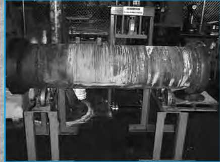
LM 2500 gas turbine coupling before being refurbished
